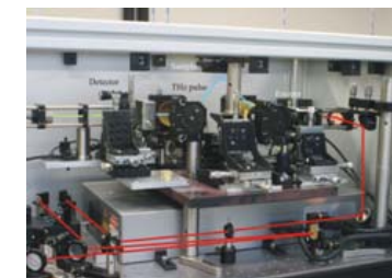
Figure 17: Photograph of the assembled scanner system: (a) complete system consisting of scanner box and instrument rack; (b) close-up view of the optical arrangement: the paths of laser beams are shown as red lines.
