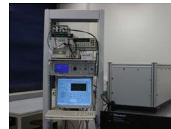
Figure 17: Photograph of the assembled scanner system: (a) complete system consisting of scanner box and instrument rack; (b) close-up view of the optical arrangement: the paths of laser beams are shown as red lines.
