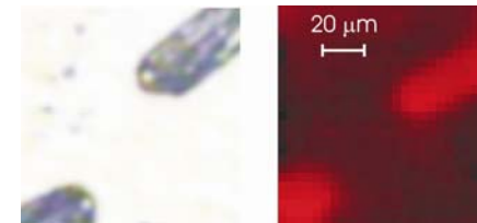
Figure 21: Visible light photograph (left) and THz image (right) of a CsI crystal
